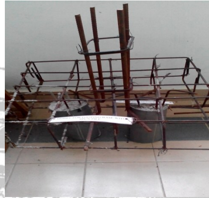
Reinforcement Pile Cap with Piling
