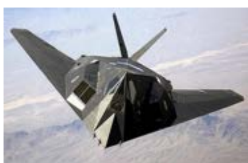
Figure 1 : F-117 Nighthawk Aircraft incorporates Stealth technology to avoid radar detection.
