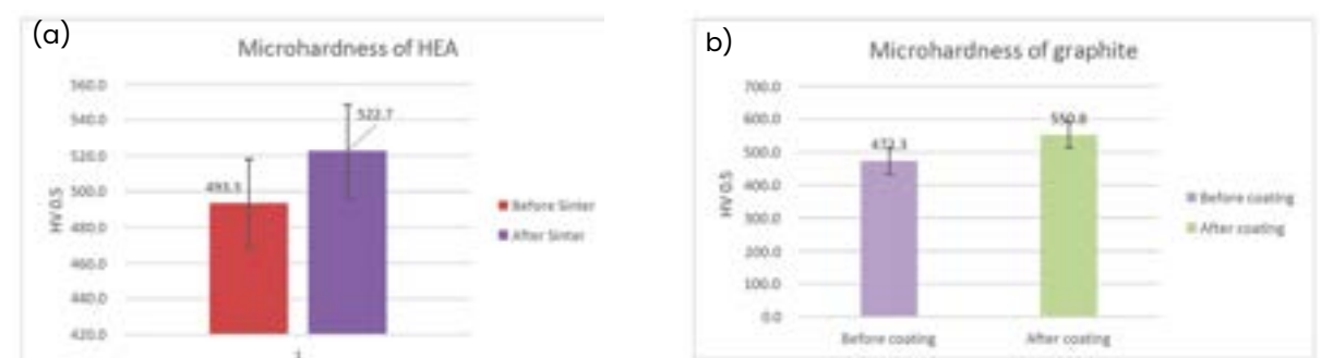
Figure 5 : (a) Microhardness test of FeCoNiAlBSi HEA powder before and after sintering at 900C and (b) microhardness of graphite before and after coating
