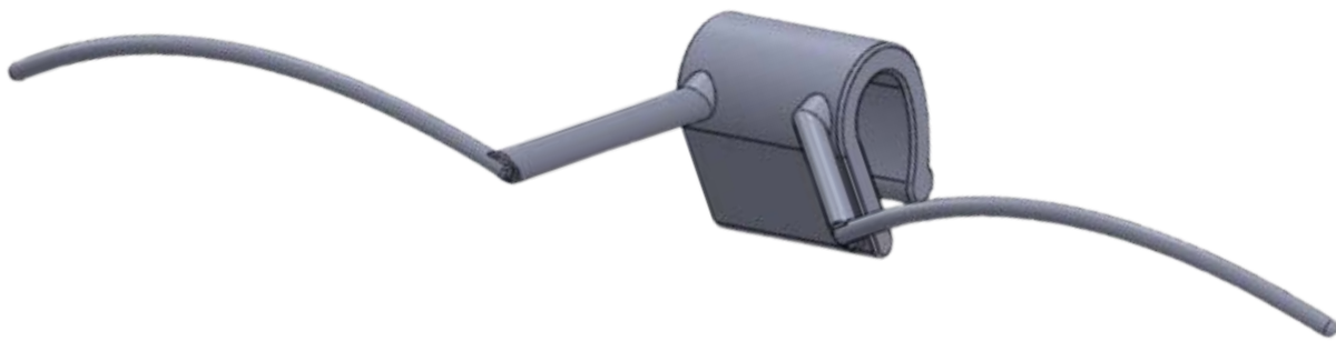
Figure 4: 3D drawing design of our crutch by using TPU material
