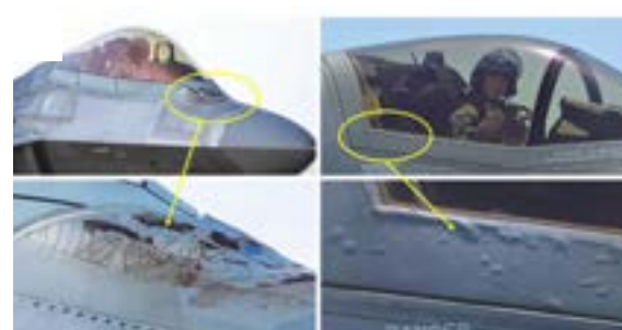
Figure 2 : Void and cracks phenomena in stealth coating on F22 [1].
