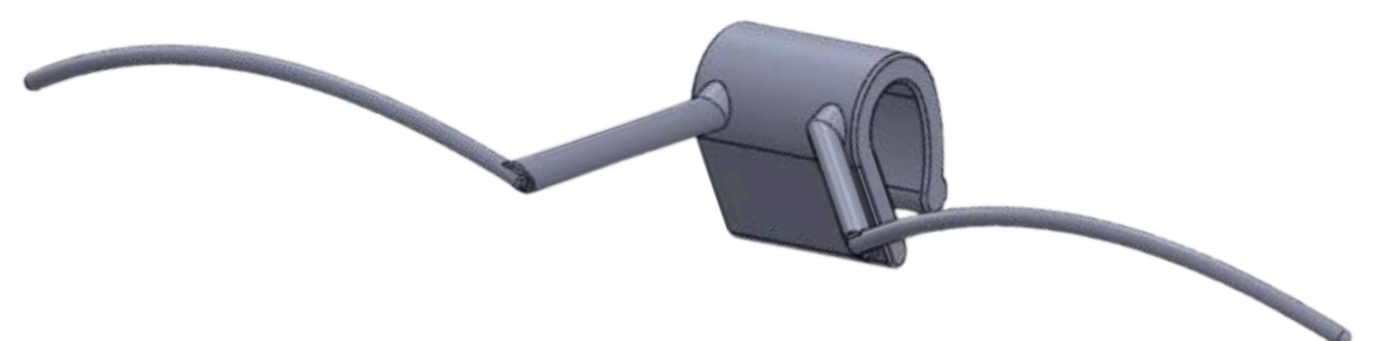
Figure 4: 3D drawing design of our crutch by using TPU material
