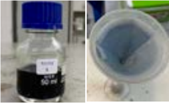
Fig 6. Stable dispersion - No sedimentation after being left for 20 days and less agglomeration
